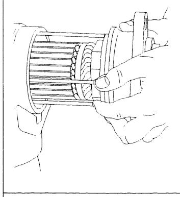
Disassembling engaging shaft
